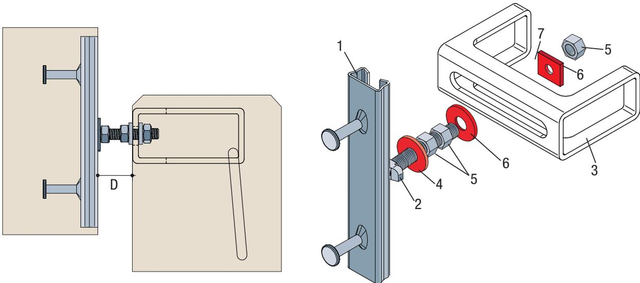
In case of distanced restraint, the distance 'D' is determined by the customer, on the specific application. The minimum length of the Bolt 'L' is determined on the base of the Distance 'D' to be produced and the type of the profile to be used.
