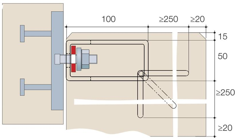
**In case of narrow or thin elements, be sure to supply for a reinforcement which is NOT INFERIOR to the one previously mentioned.**
